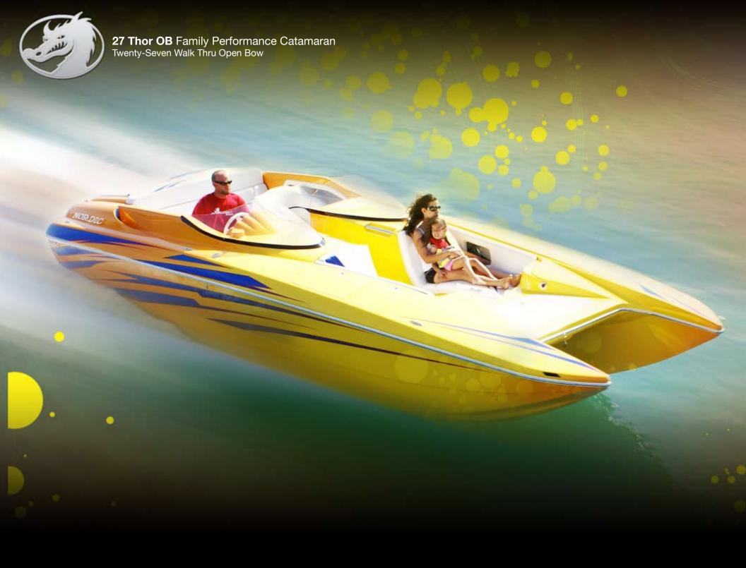
Overall boat length......27' 2" Beam length......103" Approximate weight ......4,000 lbs Fuel capacity.....90 Gallons Deadrise at transom......N/A
