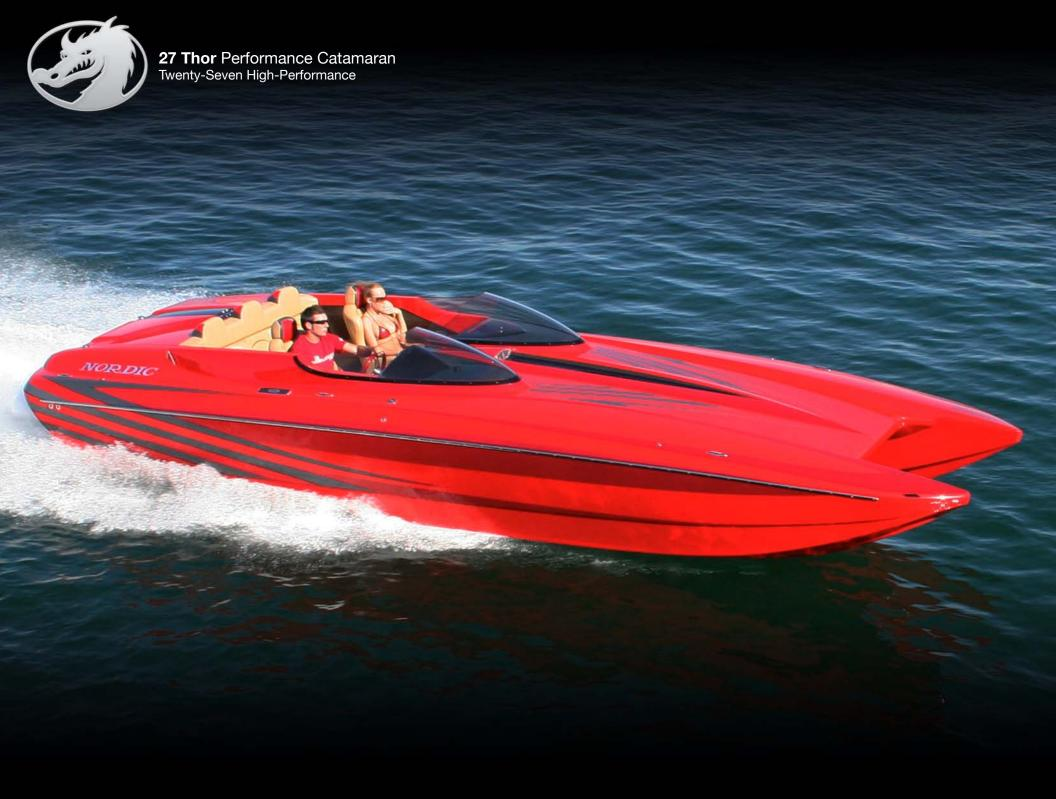
Overall boat length.....27' 2" Beam length......103" Approximate weight ......4,000 lbs Fuel capacity......90 Gallons Deadrise at transom......N/A
